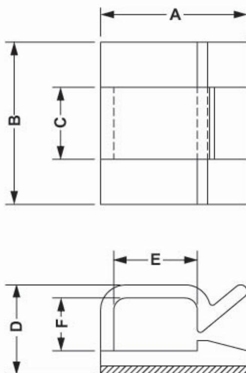
**SPESORE ADESIVO / ADHESIVE THICKNESS: 1.1 mm**
